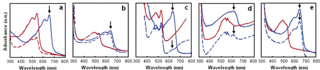
**Figure 3.** UV-vis spectra of the nanocomposite films subjected to a thermal cycle showing tunable chromatic reversibility. (a) S1, irreversible; (b) S2, reversible; (c) S3, partially reversible; (d) S4, partially reversible; (e) S5, reversible. The solid blue line, solid red line, and dashed line represent the spectra of the nanocomposites at room temperature prior to the thermal cycle, at 90 °C, and at room temperature after the thermal cycle, respectively.
