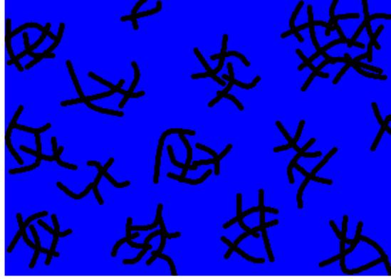
**Figure S1.** Schematic illustration of the structure for a randomly dispersed CNT/polymer composite material. The black and blue colors correspond to CNT and polymer, respectively.
