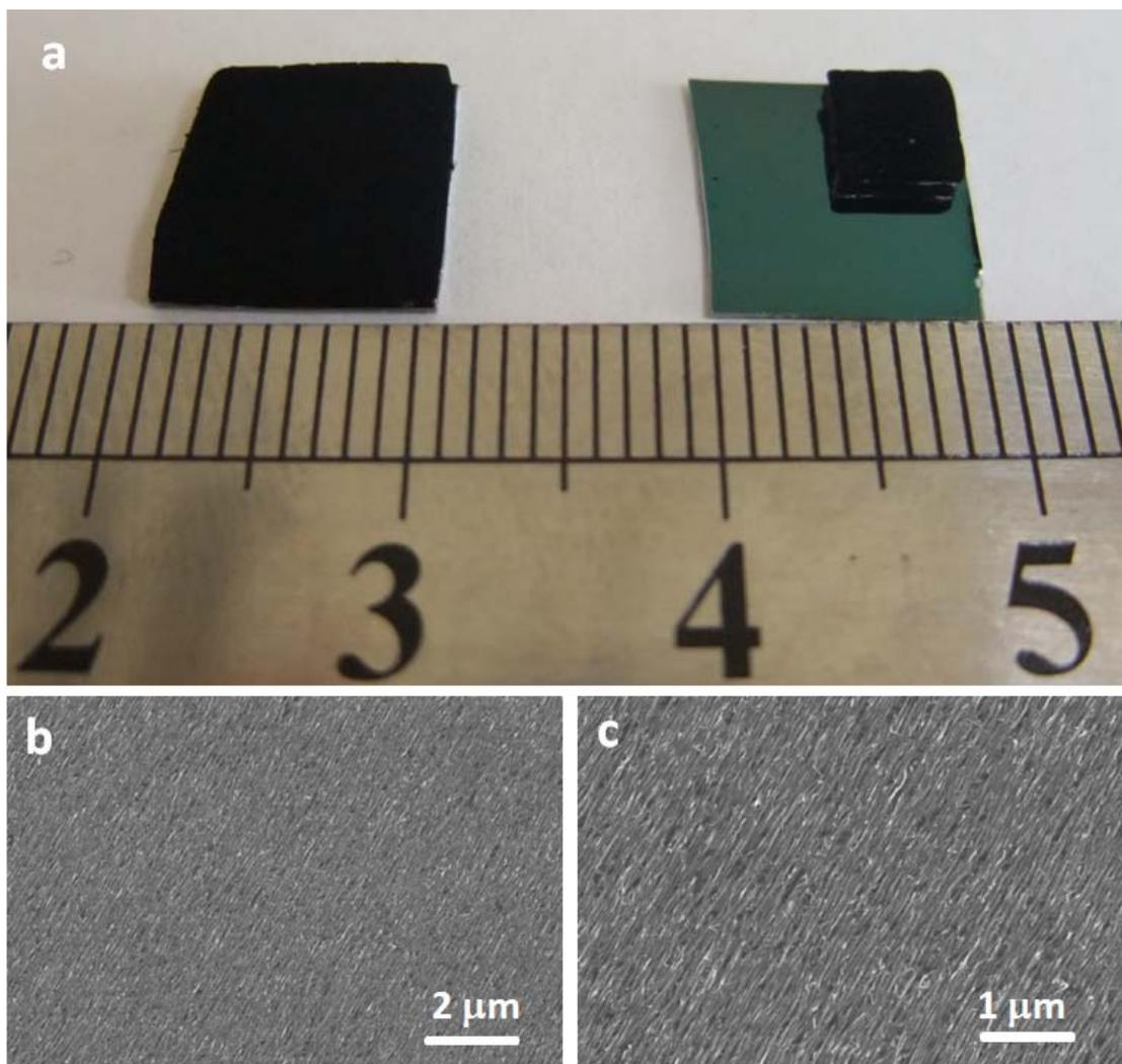
**Figure S2.** CNT densities could be greatly increased by pressing as-synthesized array from one or two sides. **a**, Photographs of a CNT array before and after being pressed. **b** and **c**, SEM images of CNT/resin film derived from the pressed CNT array.
