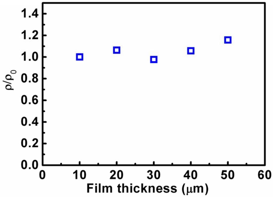
**Figure S5.** In-plane electrical resistivities of CNT/resin films with different thicknesses at room temperature. Here  $\rho_0$  and  $\rho$  are electrical resistivities of composite films at the reference thickness of 10  $\mu\text{m}$  and of other thicknesses, respectively.
