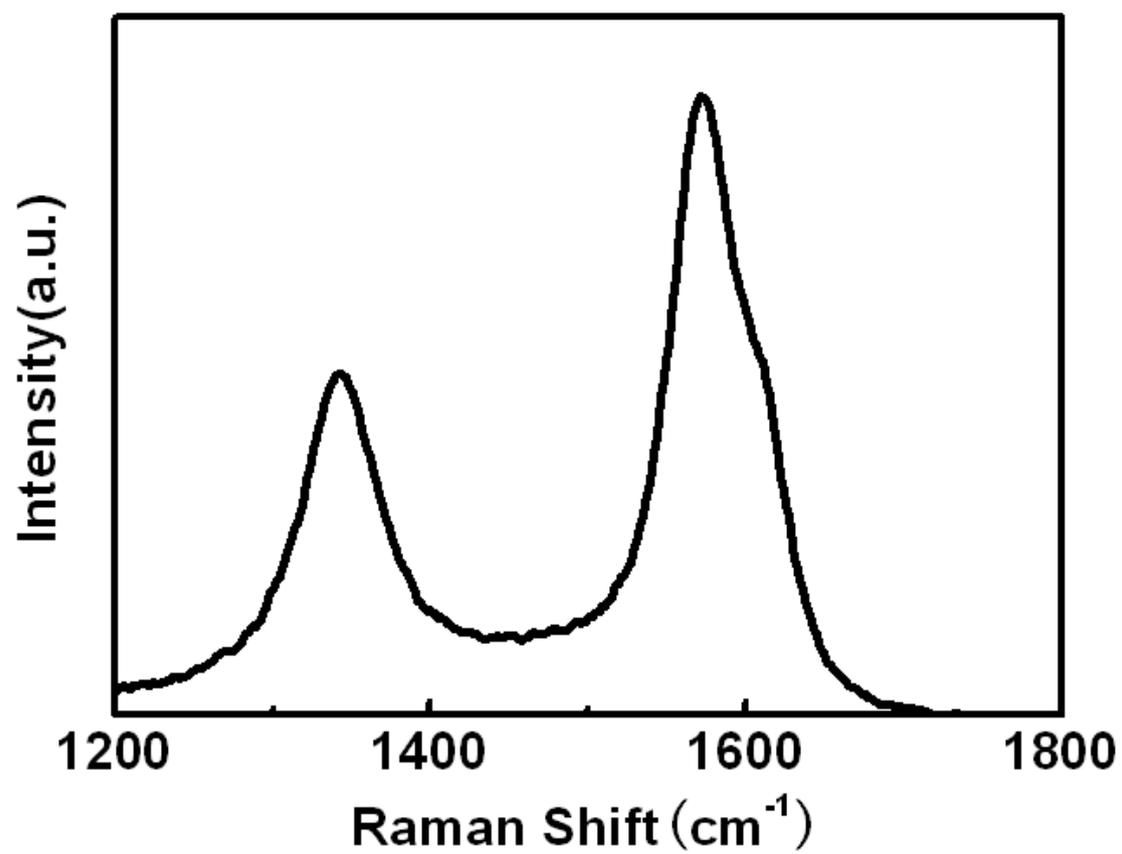
**Figure S6 .** A typical Raman spectrum of CNTs.
