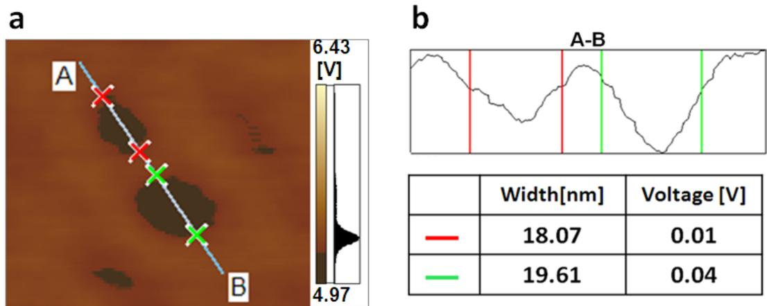
**Figure S3.** AFM image by top view of a vertically aligned and penetrated CNT/resin film.
