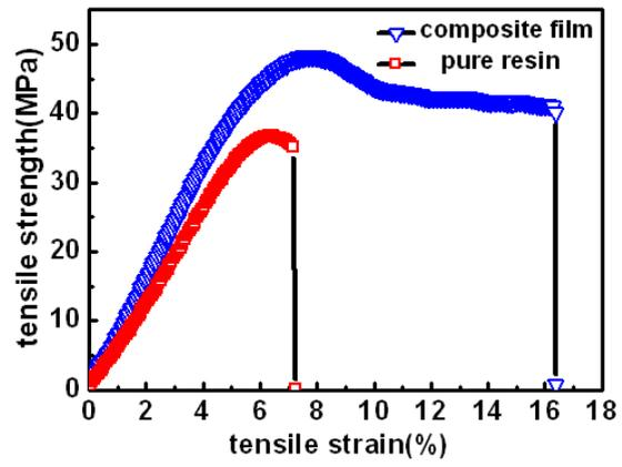
**Figure S4.** A comparison for stress-stain curves of pure resin and vertically aligned CNT/resin films in the horizontal direction.
