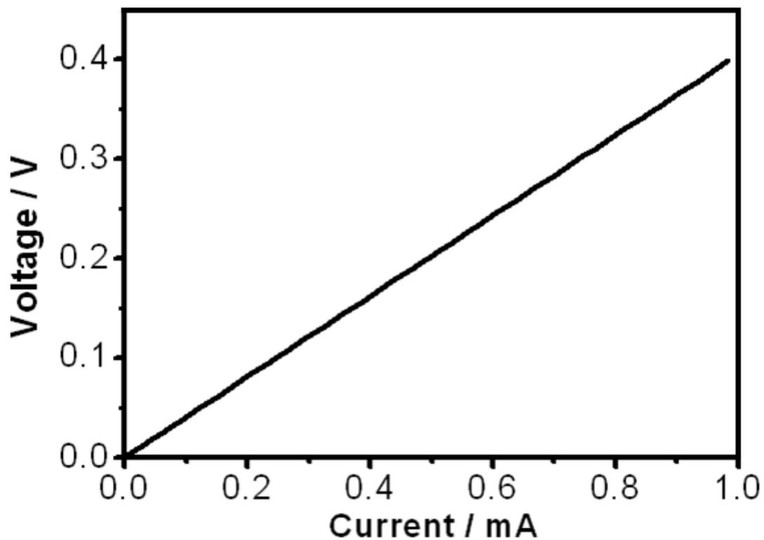
**Figure S15.** A typical I-V curve of a CNT fiber at room temperature. The fiber has a diameter of 10.5  $\mu\text{m}$  and a length of 3.5 mm. The electrical conductivity is calculated as 400 S/cm.
