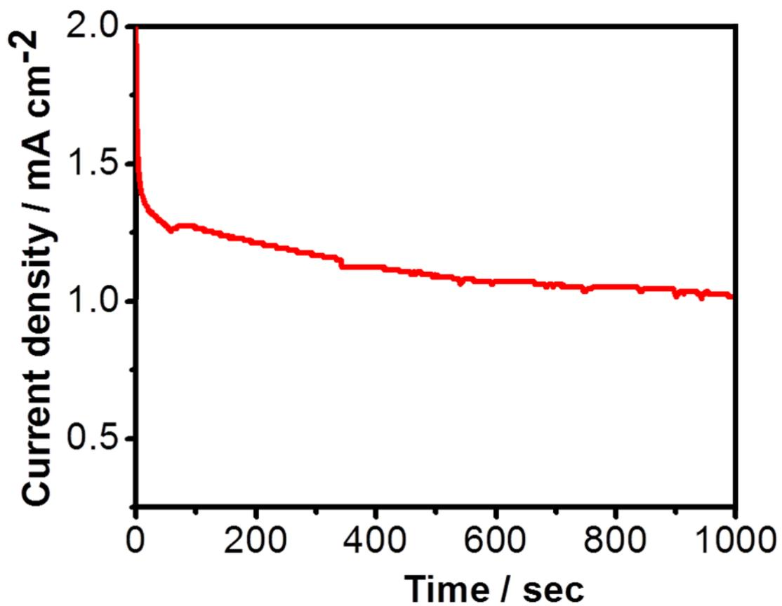
**Figure S12.** The *i-t* chronoamperometric responses of composite NCNT fiber at  $-0.25$  V in  $0.1$  M  $O_2$ -saturated KOH solution in  $1000$  s.
