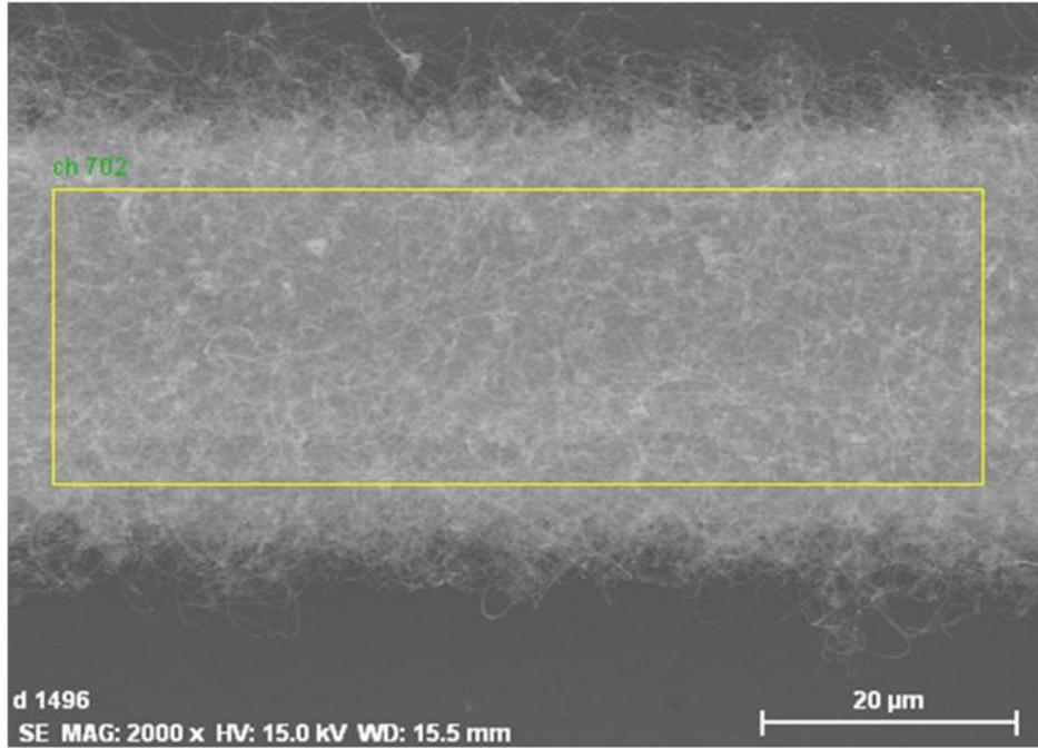
**Figure S5.** SEM image of a typical area used for energy-dispersive X-ray spectroscopy analysis of composite fiber.
