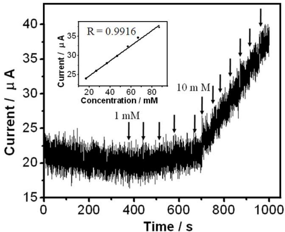
**Figure S13.** Current–time curve of CNT fiber electrode for successive addition of  $\text{H}_2\text{O}_2$  (indicated by arrows with marked concentration) to 50 mM phosphate buffered saline solution (pH of 7.4) at +0.30 V vs Ag/AgCl. Inset: calibration curve shows the linear electrode response to  $\text{H}_2\text{O}_2$  addition with correlation efficient of 0.9916.
