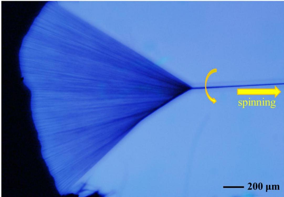
**Figure S1.** Optical micrograph of the spinning process to obtain a CNT fiber from a CNT array through a rotating probe. The left curved arrow shows the rotating direction during the spinning.
