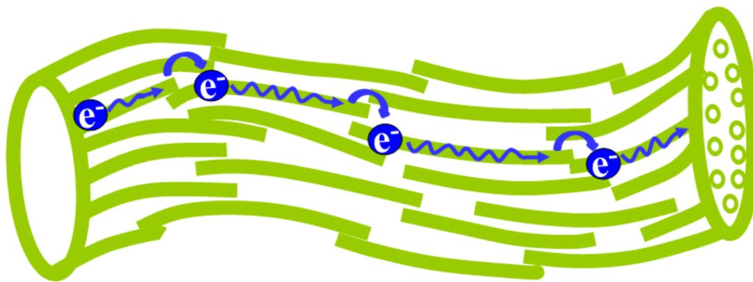
**Figure S8.** Schematic illustration of the electron transportation in local area of a CNT fiber.
