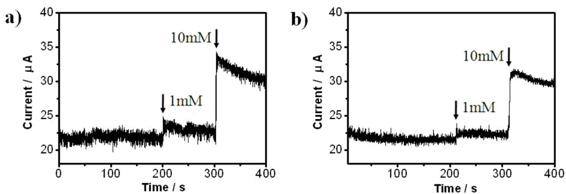
**Figure S14.** Current-time curves of a NCNT composite fiber in 50 mM phosphate buffered saline solution (pH of 7.4) after successive addition of 1 and 10 mM  $\text{H}_2\text{O}_2$  at +0.3 V at the first (a) and fifth (b) cycles. One cycle was realized after alternate sensing and washing operations of NCNT composite fiber.
