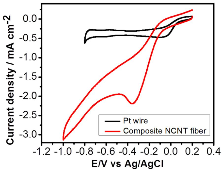
**Figure S11.** Cyclic voltammograms of the ORR for the composite NCNT fiber (red line) and platinum wire (black line) in 0.1 M O<sub>2</sub>-saturated KOH aqueous solution with the same scan rate of 100 mV s<sup>-1</sup>.
