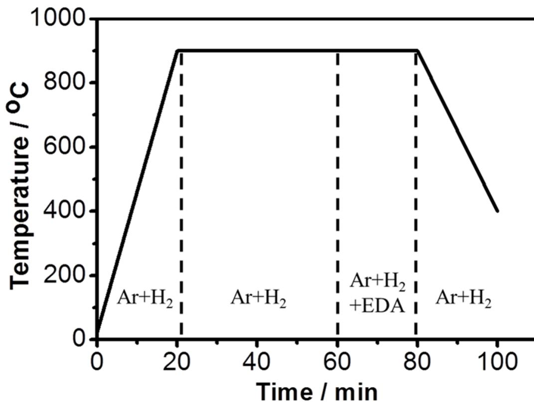
**Figure S3.** Temperature distribution during the growth of NCNTs (EDA represents ethylenediamine).
