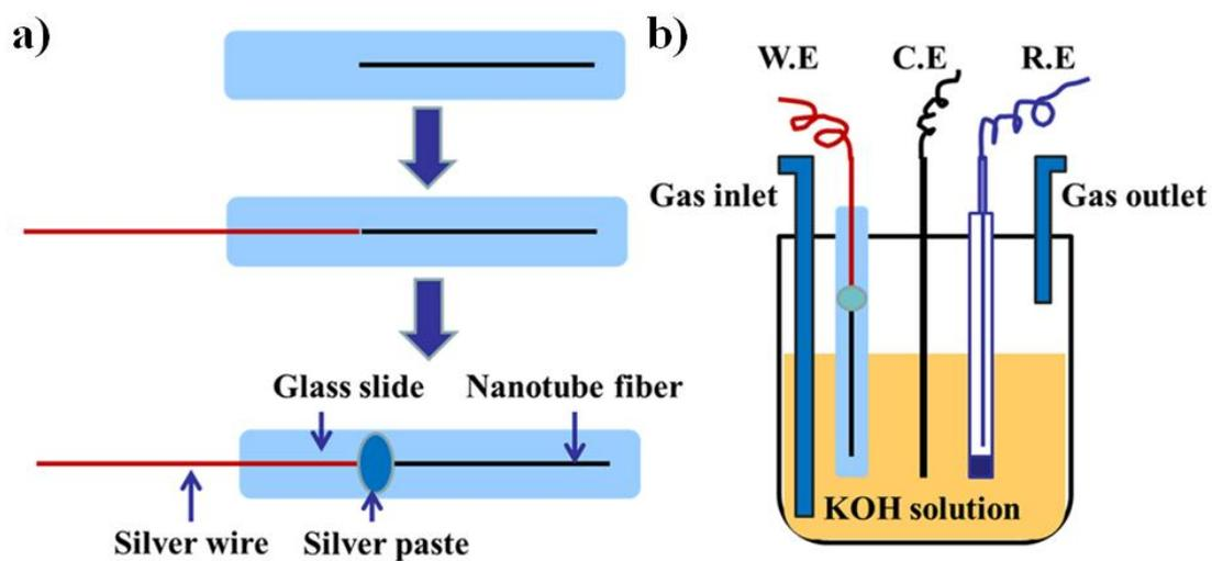
**Figure S9.** a) Schematic illustration for fabrication of a pure CNT or composite fiber as working electrode for electrochemical characterization; b) Schematic illustration for a three-electrode system using a pure CNT or composite fiber as working electrodes (W.E), platinum wire as counter electrode (C.E), and Ag/AgCl as reference electrode (R.E).
