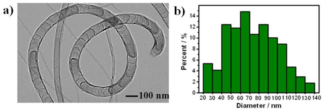
**Figure S4.** a) TEM image of NCNTs; b) The diameter distribution of NCNTs calculated from TEM images. Note that the smaller linear CNTs at a are undoped CNTs coming for the core part of composite fiber.
