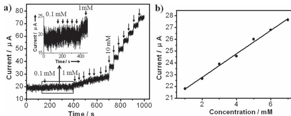
**Figure 5.** Composite NCNT fiber as an electrode for the sensitive detection of  $H_2O_2$ . a) Current–time curve of a composite fiber electrode with successive addition of  $H_2O_2$  (indicated by arrows with marked concentrations) to a buffer solution at  $+0.30 \text{ V}$  versus Ag/AgCl. b) Linear relationship between the current of the fiber electrode and the concentration of added  $H_2O_2$  (correlation coefficient of 0.9937).
