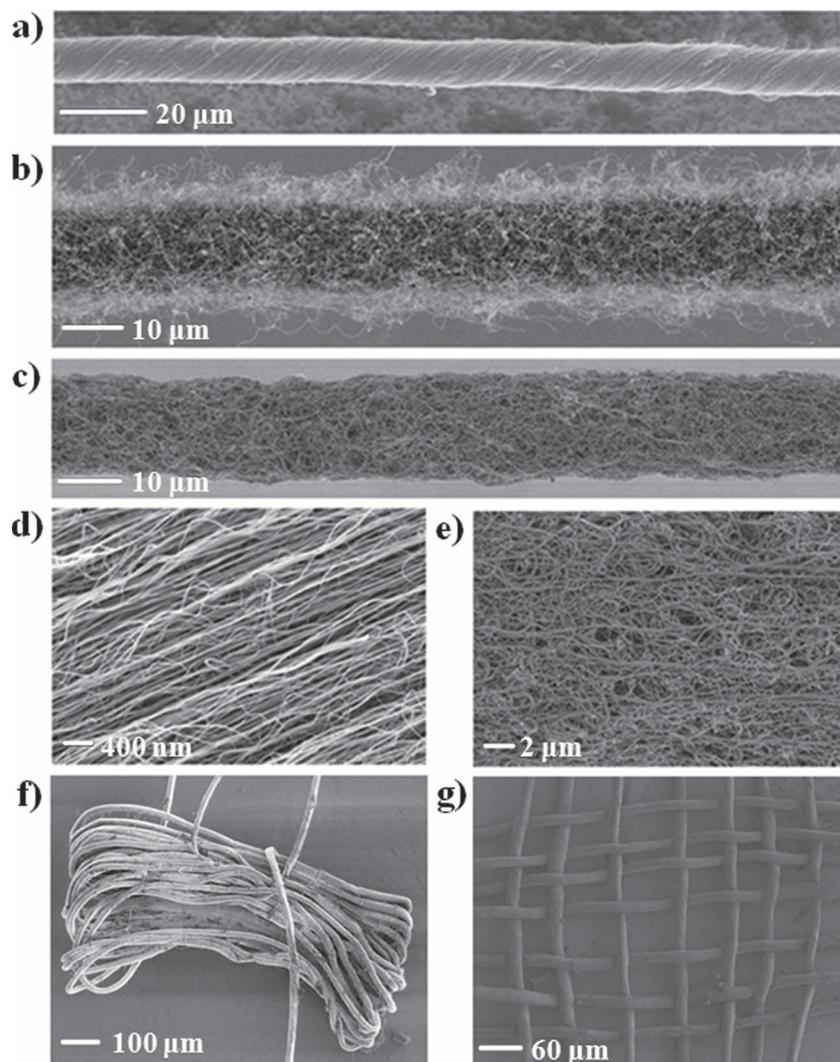
**Figure 1.** SEM images of undoped CNT and composite NCNT fibers. a) An undoped CNT fiber. b) An as-synthesized composite NCNT fiber. c) A composite NCNT fiber after being concentrated in *N,N*-dimethylformamide. d) Higher magnification of (a). e) Higher magnification of the NCNTs in (c). f) A CNT fiber being bent to form a bundle. g) A textile woven from CNT fibers.
