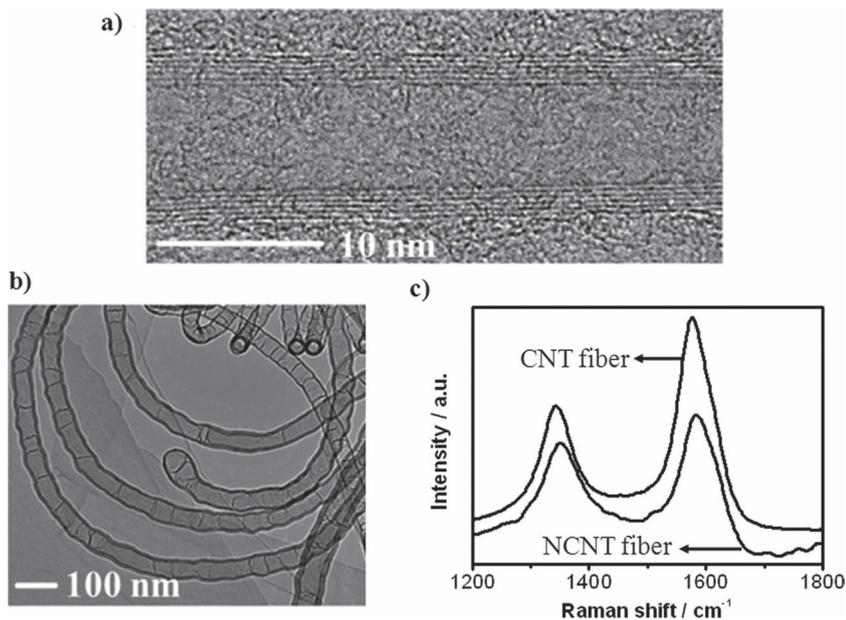
**Figure 2.** TEM and Raman spectroscopy characterization of CNTs and NCNTs. a) TEM image of a CNT. b) TEM image of NCNTs. c) Raman spectra of CNT and NCNT composite fibers.
