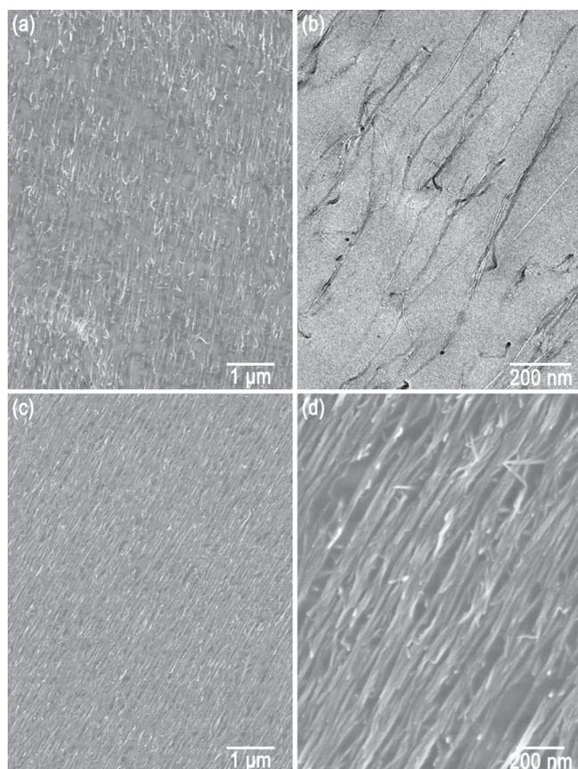
**Figure 2.** Structure characterizations of aligned CNT/epoxy films by SEM and TEM. a,b) SEM and TEM images, respectively, of the aligned CNT/epoxy film derived from an as-synthesized CNT array. c,d) SEM images of the aligned CNT/epoxy film derived from a pressed CNT array (improved three times in CNT density) at low and high magnification, respectively.
