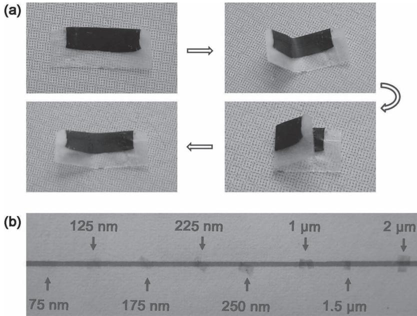
**Figure 3.** Photographs of aligned CNT/epoxy films. a) Good flexibility of a composite film, which is bent without breaking. b) High transmittances of composite films with different thicknesses.
