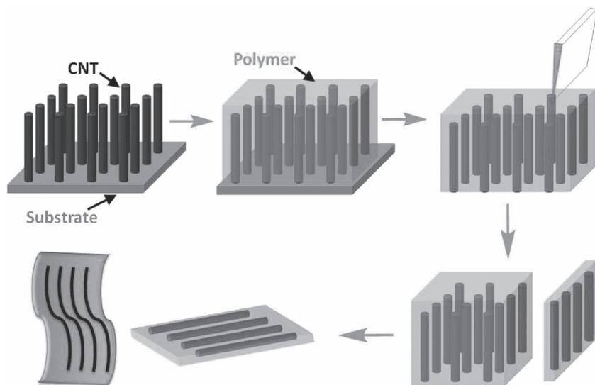
**Figure 1.** Schematic illustration to the fabrication of the aligned CNT/polymer composite film.
