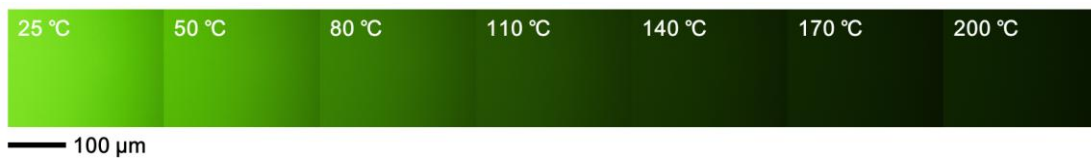
Figure S8. Fluorescent micrographs of a pure PTP film being heated to different temperatures.
