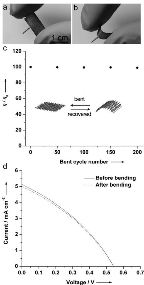
**Figure 4.** a, b) and b) Photographs of the PSC textile before (a) and after (b) bending. c) Dependence of the energy conversion efficiency of the PSC textile on the bending cycle.  $\eta_0$  and  $\eta$  correspond to the energy conversion efficiencies before and after bending, respectively. d)  $J$ - $V$  curves of the PSC textile before and after bending for 200 cycles.
