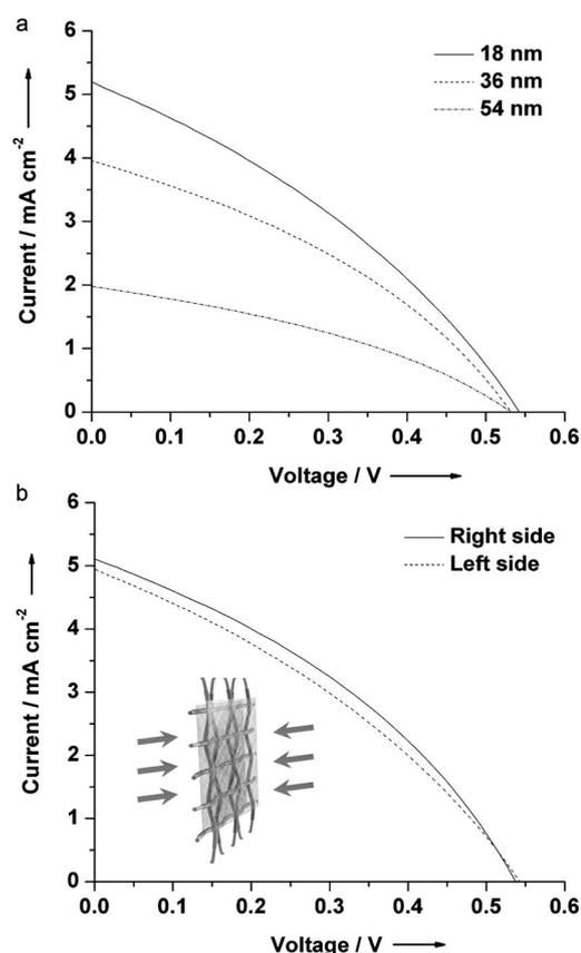
**Figure 3.** a)  $J$ - $V$  curves of the PSC textiles with an increase in the thickness of the aligned CNT sheets from 18 to 36 to 54 nm. b)  $J$ - $V$  curves of a PSC textile with an aligned CNT sheet with a thickness of 18 nm.
