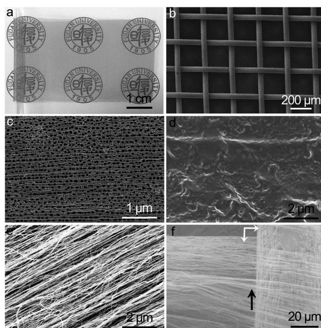
**Figure 2.** a) Photograph of a Ti textile with one part wrapped around a glass rod and the other part on a labelled paper. b) SEM image of the Ti textile. c) SEM image of aligned  $\text{TiO}_2$  nanotubes. d) Layers that were coated with P3HT:PCBM and PEDOT:PSS. e) Aligned CNT sheet. f) Aligned CNT sheet closely attached to the surface of the Ti textile. The white arrows indicate two crossed Ti wires while the black arrow indicates an aligned CNT sheet.
