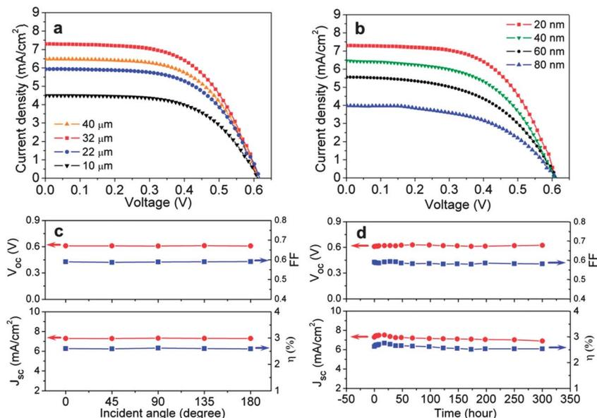
Fig. 3  $J$ - $V$  curves of the quasi-solid-state, coaxial DSC fiber. (a) Titania nanotubes with different lengths. (b) MWCNT sheets with different thicknesses. (c) Dependence of the photovoltaic parameters on the incident angle. (d) Changes of photovoltaic parameters during a period of 300 hours.
