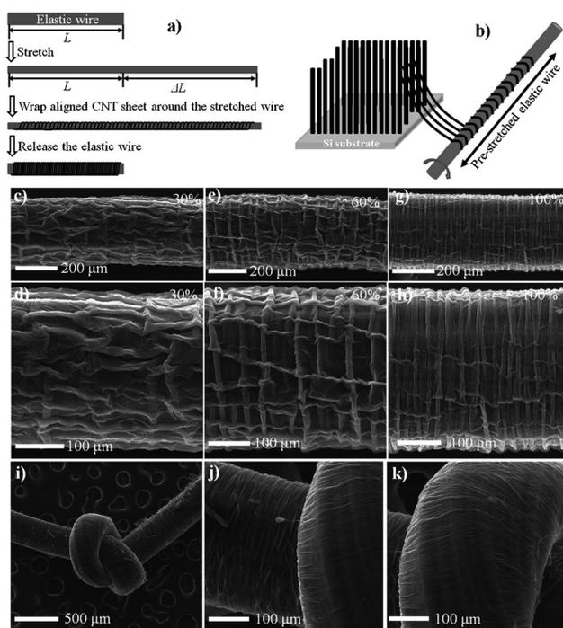
**Figure 1.** a,b) Schematic illustration of fabricating stretchable conducting wire by wrapping aligned CNT sheet around a pre-stretched elastic wire. Morphology and flexibility of the CNT-wrapped 64% polyester and 36% polyurethane elastic wire. SEM images of the buckled CNTs wrapped on the elastic wire with a 30% (c,d), 60% (e,f), and 100% (g,h) pre-strain. i–k) SEM images of a knot made from the CNT-wrapped elastic wire with a 100% pre-strain.
