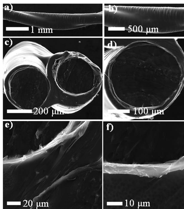
**Figure 2.** a,b) Top-view SEM images of the wire-shaped supercapacitor with a twisted structure under different magnifications. c,d) Cross-section SEM images of the twisted wire-shaped supercapacitor under different magnifications. e,f) Enlarged views of the region between the two twisted electrodes showing the electrolyte coating and CNT layers.
