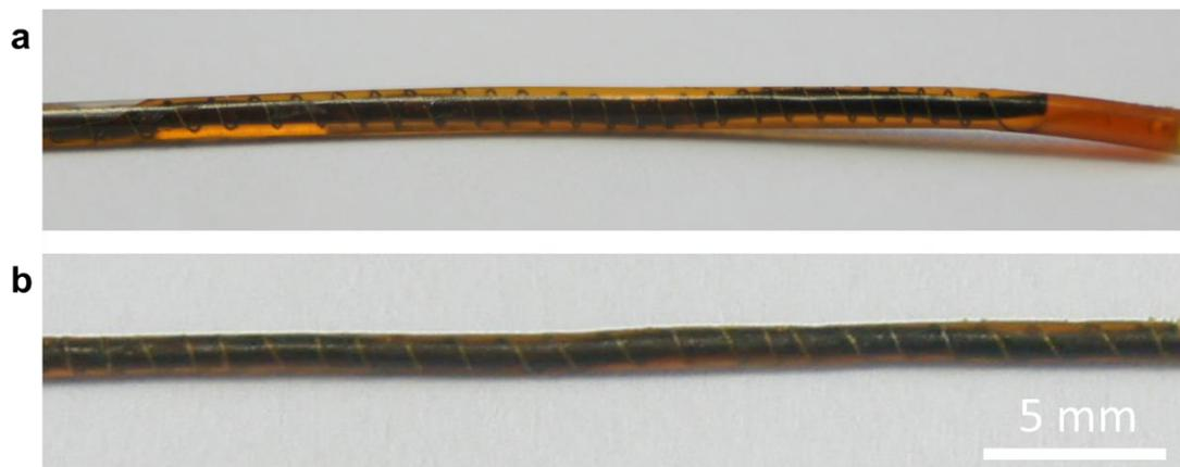
**Figure S3.** Dye-sensitized solar cells (DSSCs) fabricated from the IL gel electrolyte with (a) and without (b) encapsulation.
