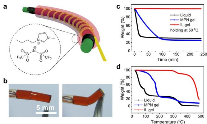
**Figure 1.** a) Schematic illustration to the structure of a stretchable fiber-shaped dye-sensitized solar cell (DSSC) and the chemical components of ionic liquid (IL) gel electrolyte. b) Photographs of IL gel electrolyte under natural and bending states. c) Weight losses of three different kinds of electrolytes traced at the same temperature of 50 °C. d) Weight losses of three different kinds of electrolytes from room temperature to 500 °C.
