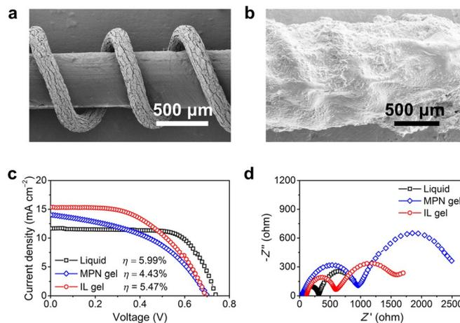
**Figure 2.** a and b) Scanning electron microscopy (SEM) images of a stretchable fiber-shaped DSSC before and after injection of IL gel electrolyte. c and d) *J*-*V* and EIS curves of stretchable fiber-shaped DSSCs based on liquid, gel, and IL gel electrolytes.
