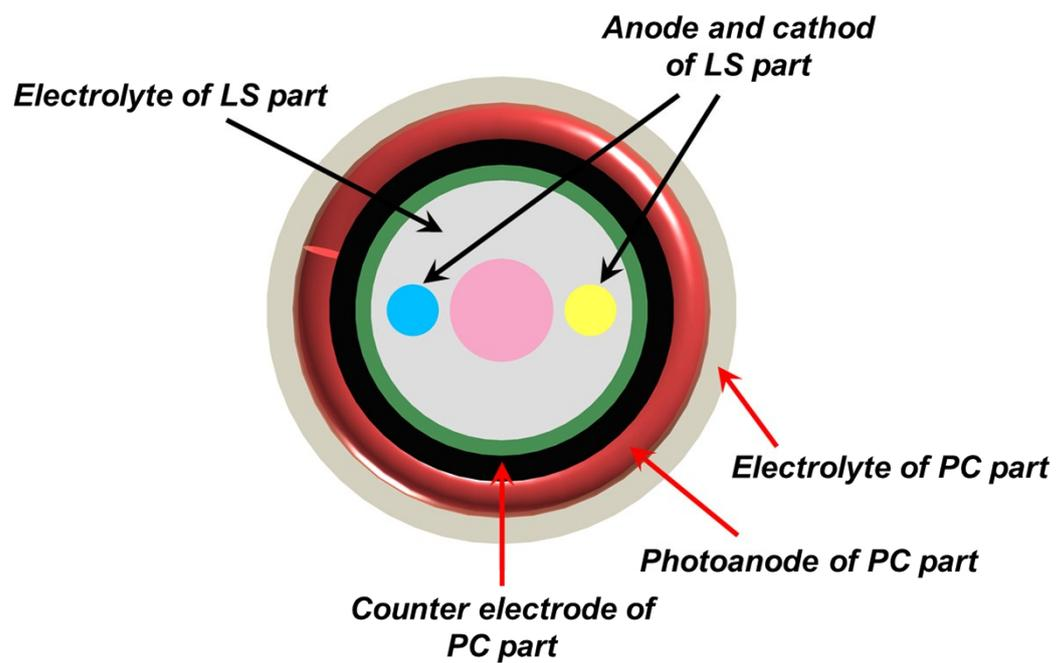
**Figure S1.** Schematic illustration to the cross-sectional structure of the FIED.
