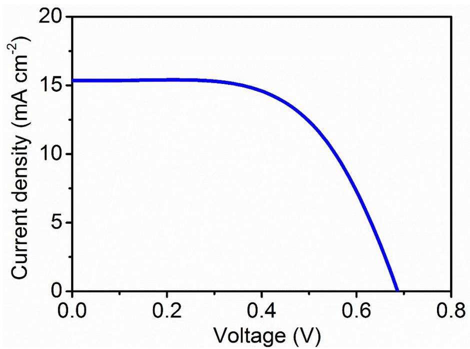
**Figure S3.** Current density-voltage curve of a photovoltaic conversion unit.
