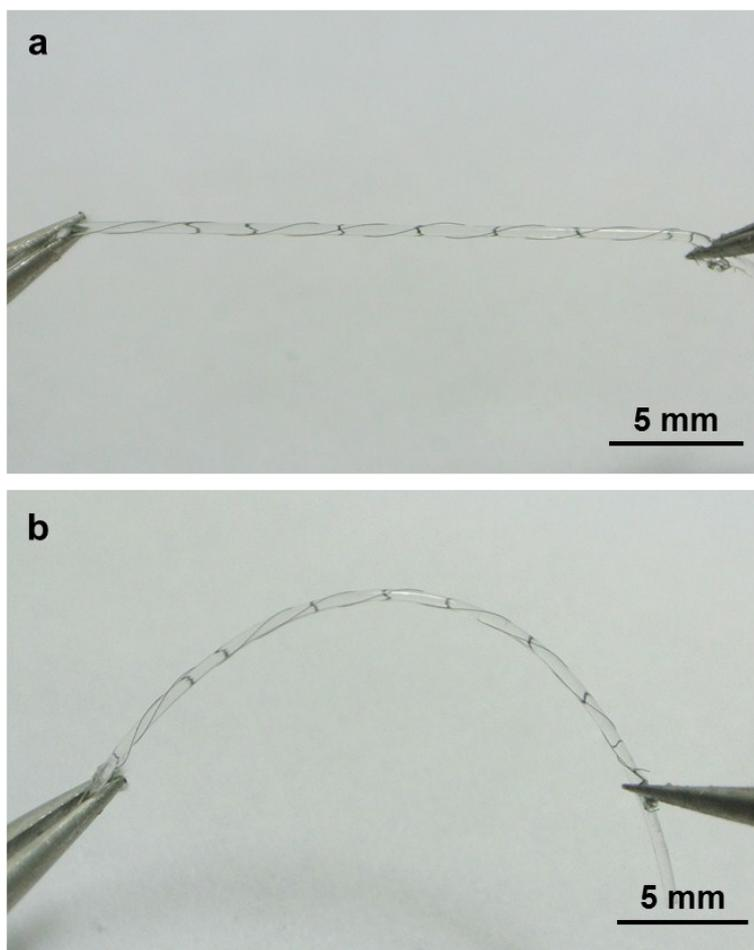
**Figure S4.** Photograph of multi-walled carbon nanotube (MWCNT)/LTO and MWCNT/LMO hybrid electrodes wrapping on a rubber fiber at original (top image) and bending (bottom image) states.
