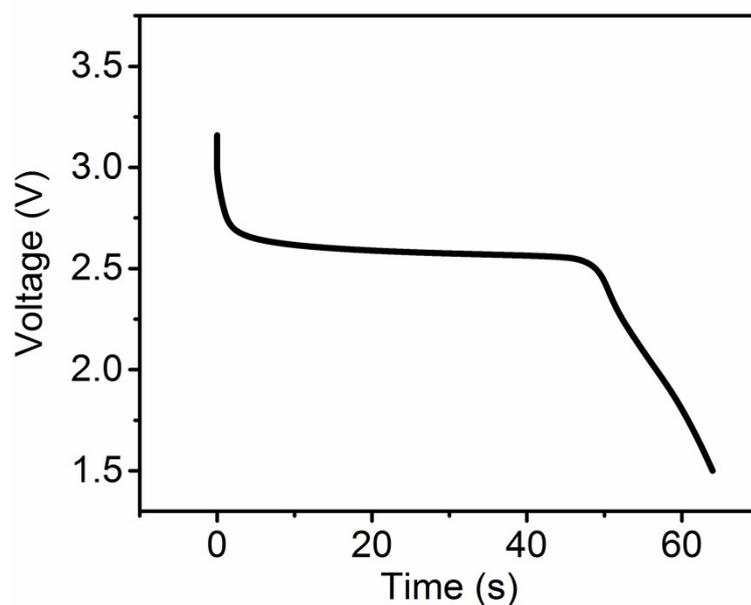
**Figure S6.** Discharging curve of an LS part with increased discharge plateau by adding amorphous carbon to MWCNT/LMO electrodes. Discharge current, 0.05 mA.
