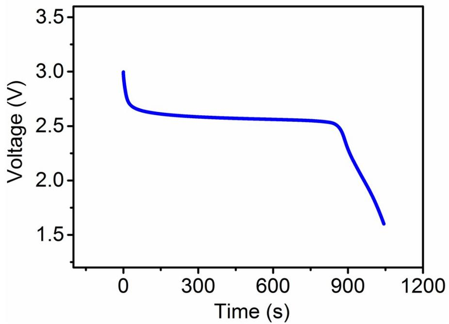
**Figure S5.** Discharging curve of an LS part with enhanced capacity by using more active materials at both fiber electrodes. Discharge current, 0.02 mA.
