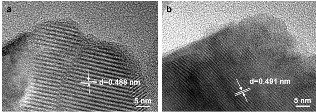
**Figure S2.** **a** and **b.** TEM images of  $\text{LiMn}_2\text{O}_4$  (LMO) and  $\text{Li}_4\text{Ti}_5\text{O}_{12}$  (LTO) nanoparticles, respectively.
