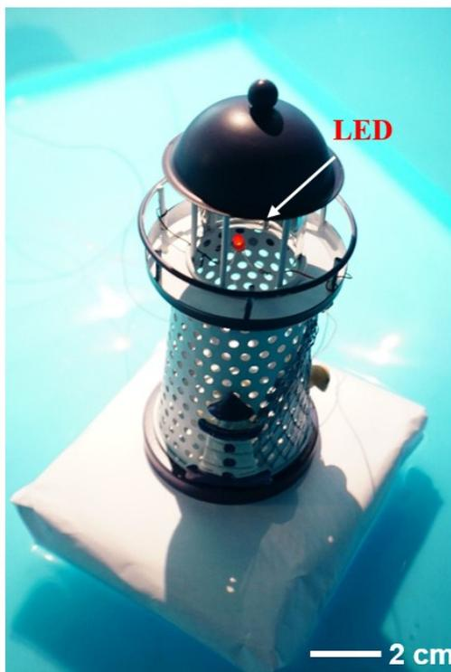
Fig. S17. Photograph of the light-emitting diode powered by ten photo-to-electricity systems connected in series.
