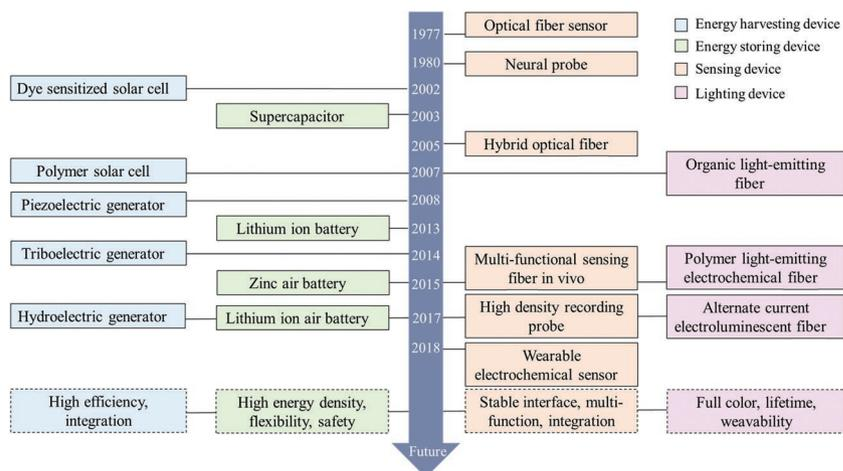
**Figure 1.** A timeline showing the advance of fiber-shaped electronic devices with regard to the four main functions: energy harvesting, energy storage, sensing, and lighting.
