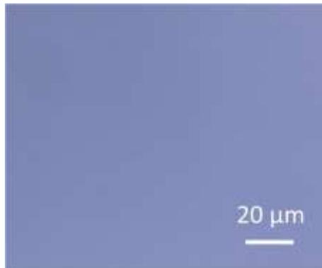
**Figure S1.** Optical image of *h*-BN film grown on SiO<sub>2</sub>/Si by PECVD (30 min).
