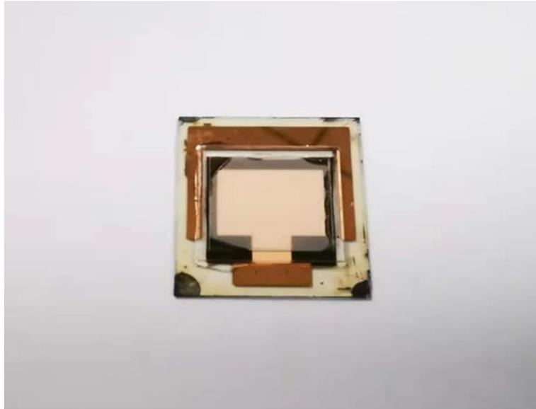
**Supporting Figure 14** | Photograph of the all-perovskite monolithic tandem photovoltaic cell with an active area of 1 cm<sup>2</sup>.
